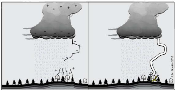
Fig. 1: A stepped leader moves down in 50m steps. Multiple streamers rise from tall objects near the leader. There are many more streamers than direct strikes.
